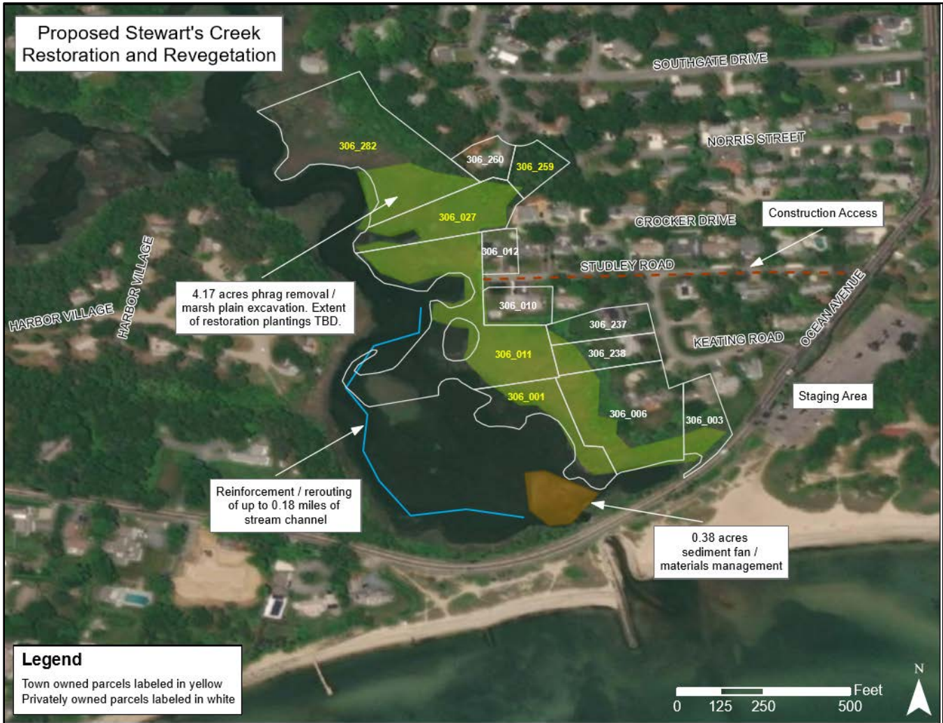
Figure 1 – Proposed project components, parcel ownership, construction access, and staging area for improvements to Stewart’s Creek.
